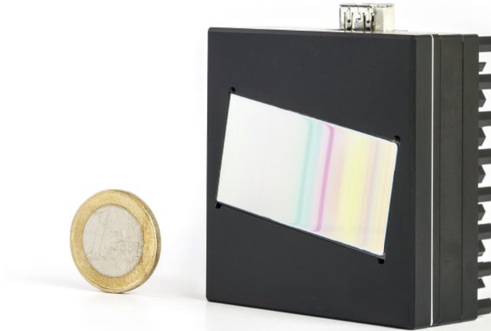
Snapshot multispectral camera demonstrator (Source all images: the authors)
